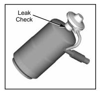
■ Insert the regulator pipe firmly. The regulator uses a push-on fitting to attach to the stove. It is necessary to hold the stove to make sure the fitting is seated. Align the regulator to the fuel tube on the rear of the stove and push on until you hear the retainer "click" in place. Gently pull on the regulator to ensure that the connection is secure.
