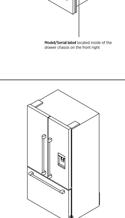
Model/Serial label located bottom right hand corner of freezer, behind freezer door
