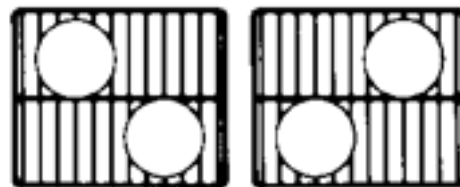
FIG. 15 PAN POSITIONING—TOP RACK (LEFT), BOTTOM RACK (RIGHT)
