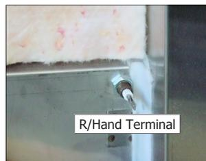
8. From inside the proofer, withdraw the element.
