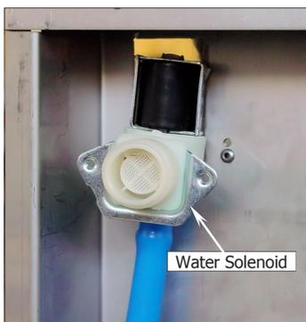
11. Refit water solenoid mounting bracket by pushing top of bracket up under top panel lid.
