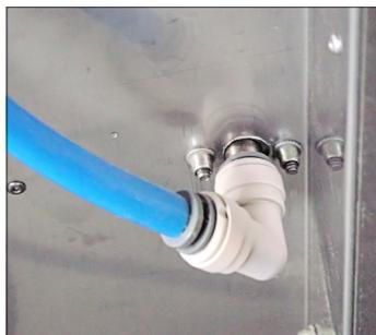
10. Insert replacement water solenoid into recess at rear of proofer.
