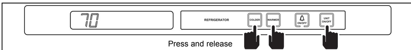
**Figure 3-74. Initiate (or Exit) Showroom Mode, Press COLDER, WARMER and UNIT ON/OFF Keys**
